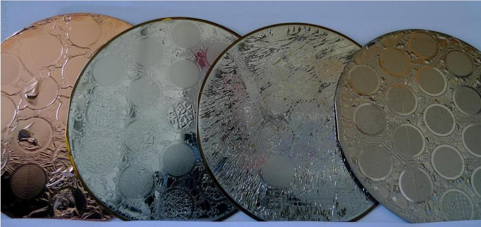
**Figure 2.8:** Picture of four wafers after metal deposition on top of SU-8. From left to right copper, titanium, chromium, titanium/tungsten were sputtered. Layers with cracks and bubbles are observed. The circles in the wafers correspond to the exposed SU-8 pattern.
