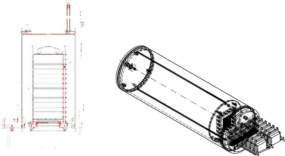
Figure 3: Examples of test TPCs as used in the R&D work. Left drawing: TPC as built by MPI Munich and used in the KEK test beam. Right drawing: TPC as built at DESY and being tested there.
