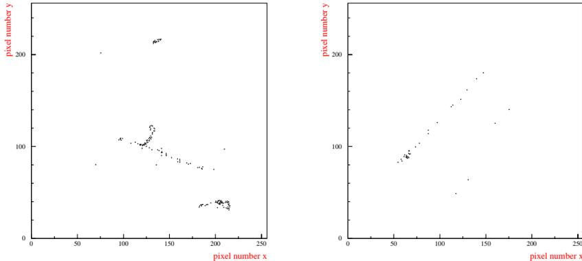
Figure 22: Left: Image recorded from the MediPix2/Micromegas prototype TPC showing a cosmic charged particle track together with a  $\delta$ -electron. The total size of the image is  $14.1 \times 14.1 \text{ mm}^2$ . Right: Image showing selected cosmic charged particle tracks.
