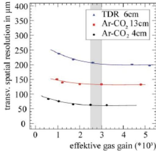
Figure 12: Point resolution as measured in a three-GEM TPC as a function of the gain.
