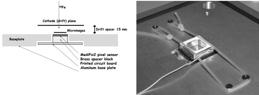
Figure 6: Left: The layout of the chamber with the MediPix2, the Micromegas and the drift gap. Right: The mounting of the Micromegas onto the MediPix2 sensor.
