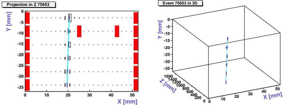
Figure 10: Event display of a single cosmic muon recorded in a 5T magnetic field with a GEM-equipped TPC; left: projection on the endplate; right: 3D view . The solid red boxes indicate dead readout pads.
