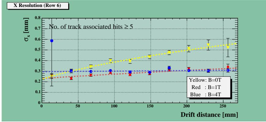
Figure 14: Point resolution measured as a function of the drift distance in a wire TPC with 1 mm sense-wire-to-pad-plane gap; 0 T and 1 T points are from test-beam data, 4 T points are from cosmics.
