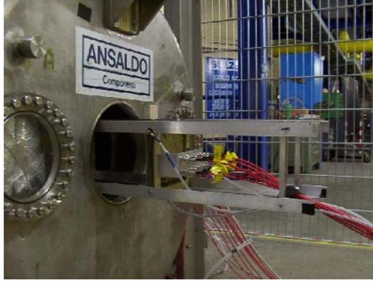
Figure 1: The 5T magnet in DESY with a test chamber inserted into the magnet bore. A 2T magnet is available at Saclay, and 1.2T/1.5T thin-walled coils are in use at KEK.
