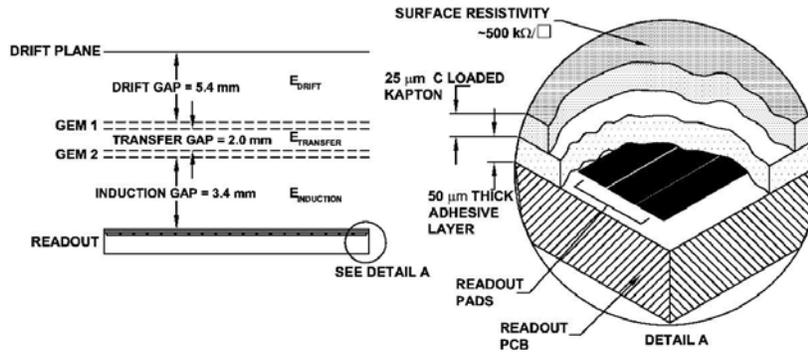
Figure 15: Schematics of the resistive anode double-GEM detector for charge dispersion studies.
