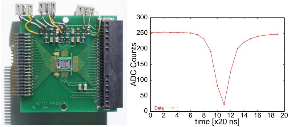
Figure 5: Photograph of the Preshape 32 chip bonded to a test board (left) and a first signal recorded with this setup
