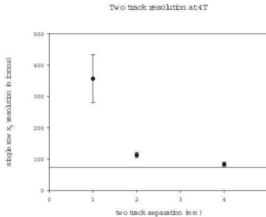
Figure 19: Single row resolution recorded in laser-induced two-track events, as a function of the separation between the two tracks. The horizontal line indicates the resolution for single laser tracks.
