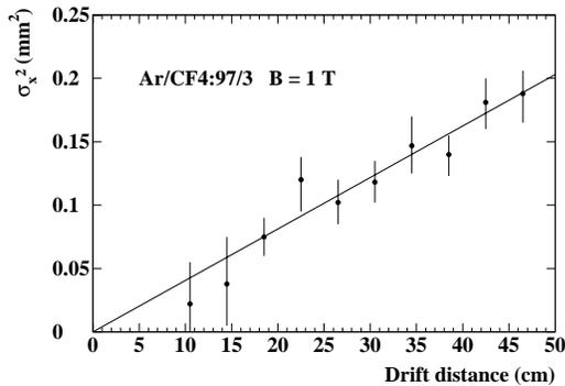
Figure 13: Track r.m.s. width measured in a Micromegas TPC at 1 T as a function of the drift distance.
