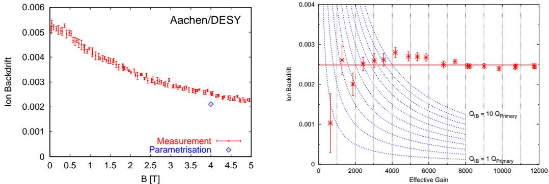
Figure 7: Left: Suppression of ion backdrift versus magnetic field. Right: Relative ion backdrift versus effective gain
