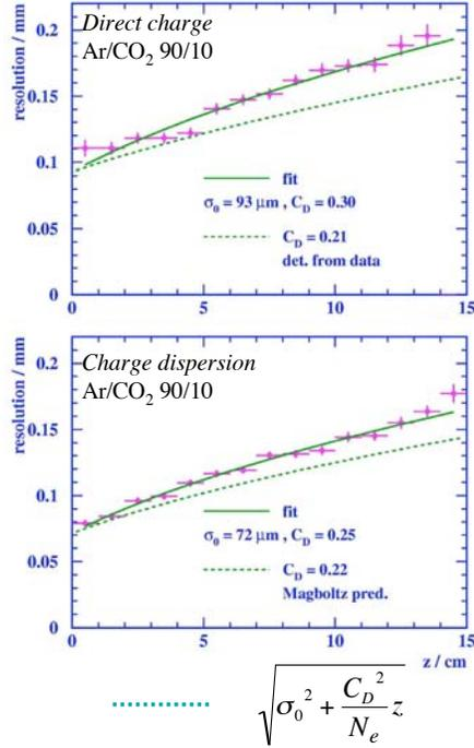
Figure 17: Charge dispersion improves TPC resolution over that from direct charge detection for low diffusion gases like ArCO<sub>2</sub>.
