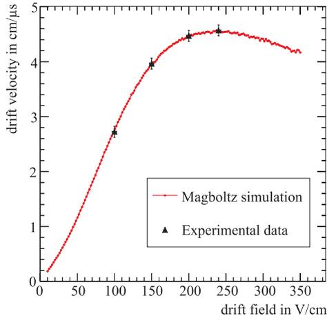
Figure 20: Drift velocity measured in the TDR gas at a fixed drift distance.
