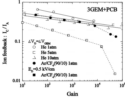
Figure 8: Ion backflow measured in a triple GEM structure, for different gas mixtures, different pressures, and as a function of the gain in the GEM system.
