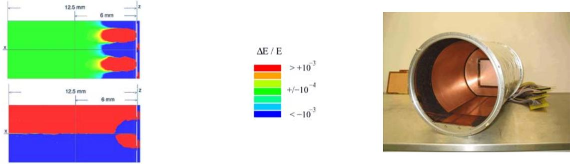
Figure 4: Left: The simulated electric field homogeneities for field cages with (top) and without (bottom) mirror strips on the outer side of the field cage. Middle: The plot on the right gives the scale of the relative deviations. Right: Photograph of the field cage.
