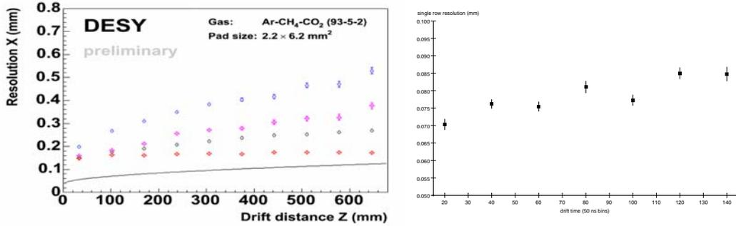
Figure 11: Point resolution measured in a GEM equipped TPC for different magnetic fields, and for different gas mixtures. Left: 93-5-2% Ar-CH<sub>4</sub>-CO<sub>2</sub> (TDR gas), right: 95-10% Ar-CH<sub>4</sub>(P10).
