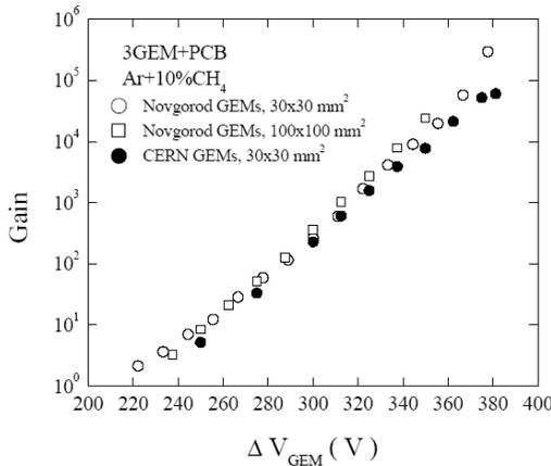
Figure 2: Gain as a function of applied voltage in triple GEM structures equipped with GEMs by different manufacturers.
