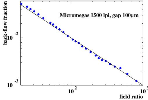
Figure 9: Ion backflow fraction as measured with Ar-10%CH<sub>4</sub>. The line is the expectation from the inverse field ratio law.
