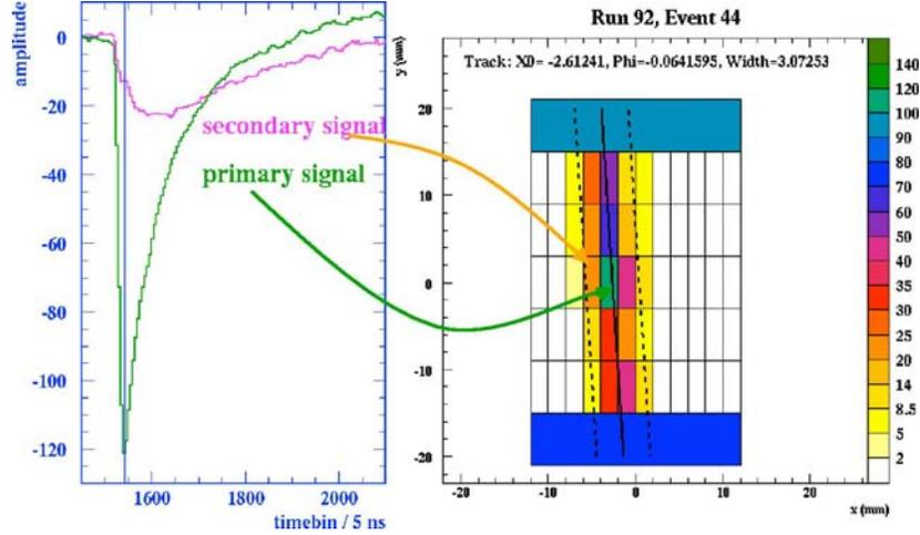
Figure 16: Charge dispersion signal on a charge collecting pad and its neighbor for a cosmic ray track in the TPC. Ar-CO<sub>2</sub>/90%-10%.
