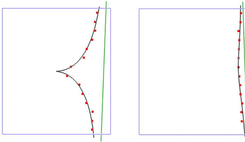
Figure 21: Distortion of tracks from cosmic ray muons with normal settings (left) and settings optimised for minimum ion backdrift (right). The charge density for these plots is about six orders of magnitude worse than expected at the ILC, and the figures are just to illustrate the improvement due to optimisation. The green line indicates the expected position of the track, if there were no distortions present. The black line is a fit to the point assuming a simple model for the distorted track.
