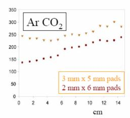
Single pad row resolution measurements from the Carleton TPC (Foil 4). Tracks are formed from the outer 6 rows, and residuals calculated for each of the two inner rows with  $2 \text{mm} \times 6 \text{mm}$  (triangles) and  $3 \text{mm} \times 5 \text{mm}$  (circles) pads. The residuals are fit to Gaussians, and the standard deviations (in microns) is shown here for different drift distances.
