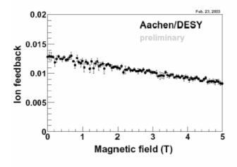
Left: the ion-feedback improves at high magnetic field in GEMs, as seen from the Aachen/DESY measurements described on Foils 10-11.
