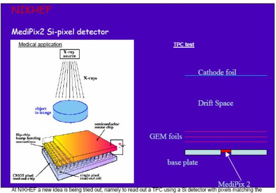
At NIKHEF a new idea is being tried out, namely to read out a TPC using a Si detector with pixels matching the GEM-hole pitch. Left: the MediPix2 chip has 256 x 256 pixels of 55 x 55 µm², low noise and a minimum threshold of about 1000 electrons. Right: schematic view of the one liter test TPC with a triple-GEM arrangement and an insert in the base plate for the MediPix2 chip.
