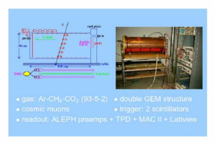
Several TPC prototypes, large and small, are now in operation. Shown here is the large one in DESY/Hamburg which uses cosmic rays to study the tracking characteristics using GEM gas-amplification. Obviously these studies are with no magnetic field. The size of the chamber is suitable for studies of gas properties and of the impact of readout geometry on the coordinate resolution.
